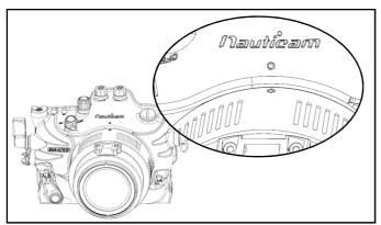
Align the mounting indices of the port and the housing; these appear as white circles on both the port and the housing.
